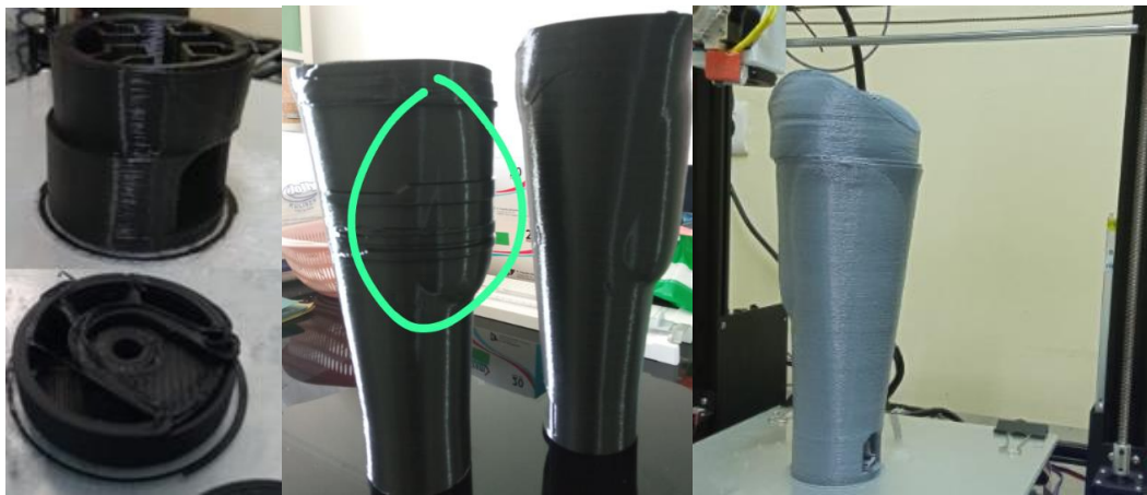
Figure 15: Examples of failed prints shared by the hospital staff
