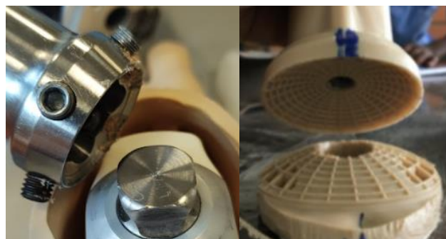
Figure 11: Ottobock Pyramid connector (left) and ICRC connector (right)
