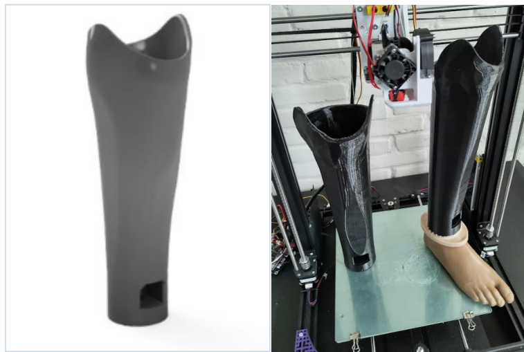
Figure 19: The final prosthesis design, digital (left) and 3D printed (right)
