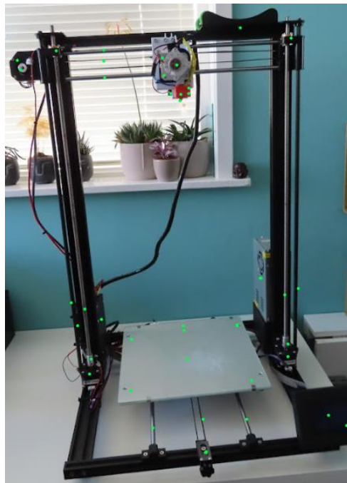
Figure 20: Critical components of the custom 3D printer, marked with green dots
