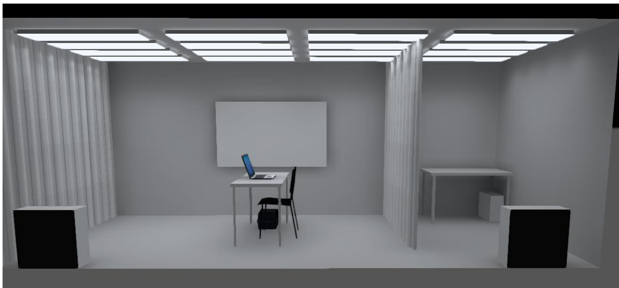
Figure 5. Side view rendering of the laboratory, showing area A (right) and area B (left) separated by a curtain (DIALux evo). Note that, in contrast to the image, the edges of the projector screen were not visible during the experiment.
