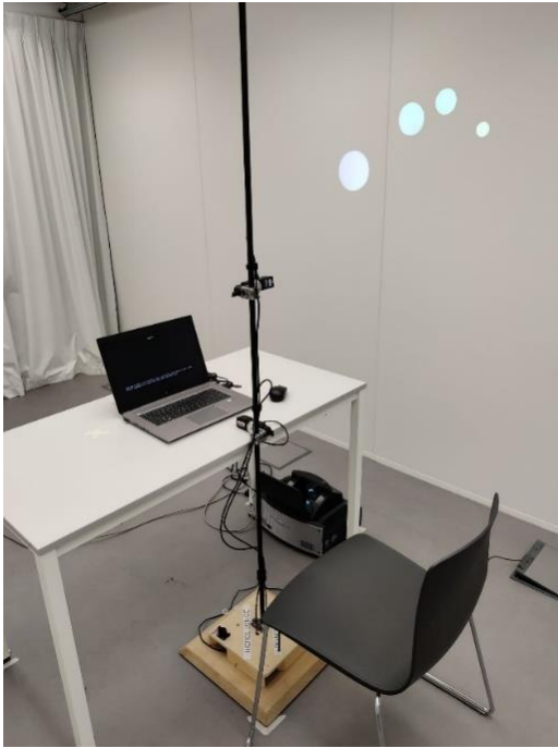
Figure 19a. Set-up of the lighting pole to perform illuminance measurements. On the right wall, the stimuli are projected.
