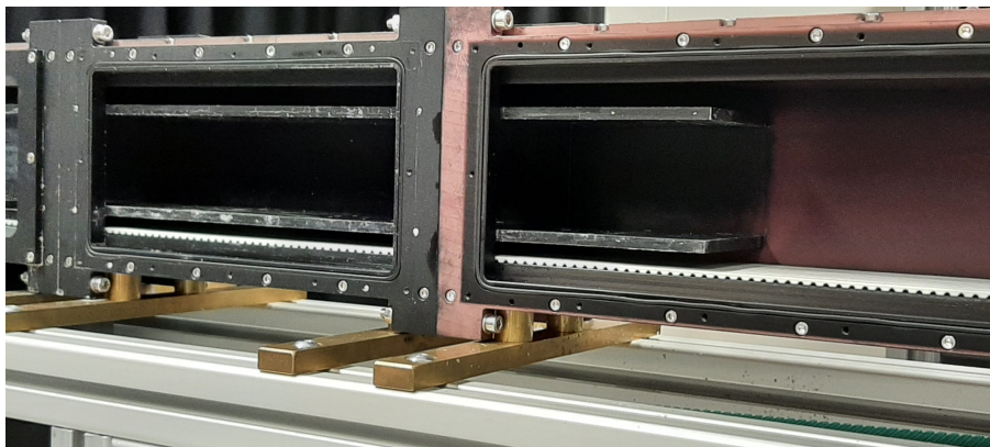
Figure 4.3: Picture of the wind tunnel with the the honeycomb and glass plate removed.
