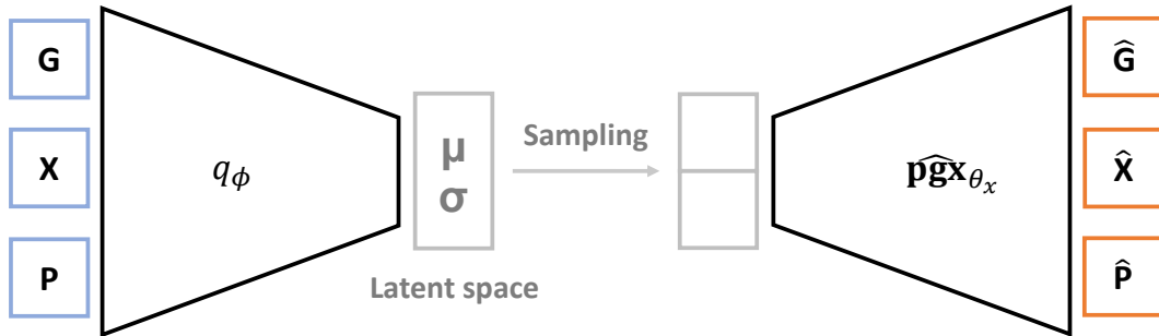
Figure 6.1: A schematic overview of Model 1.0 based on the VAE framework. The input consist of 3 categories, the Geometry data \mathbf{G} , the transport quantities \mathbf{X} and the plasma parameters \mathbf{P} . The encoder and decoder are given by q_\phi and \widehat{\text{pgx}}_{\theta_x}(\mathbf{z}) respectively.
