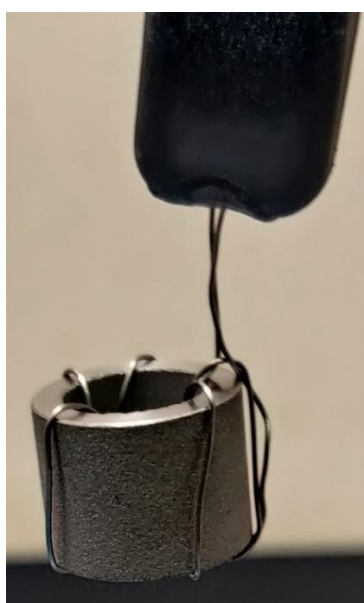
Figure 3-7 Connection for the 1 cm long porous titanium tube sample
