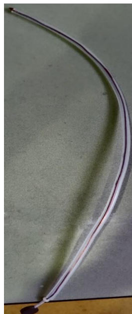
Figure 3-2 Electrical connection for the 1 and 1.5 cm diameter titanium disc samples
