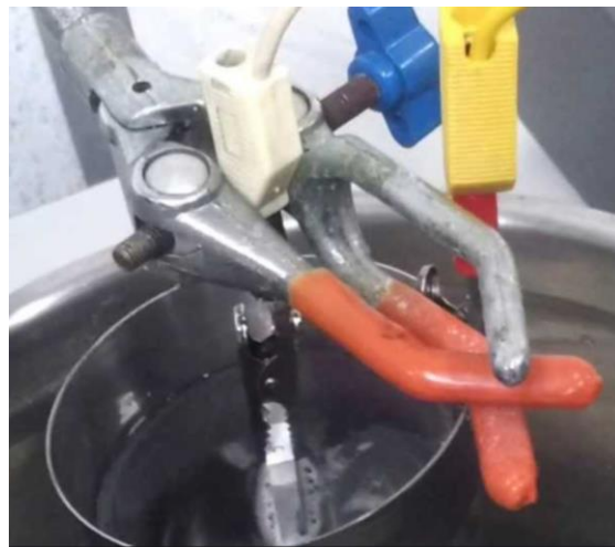
Figure 2-4 Crocodile-clip connection for larger workpieces
