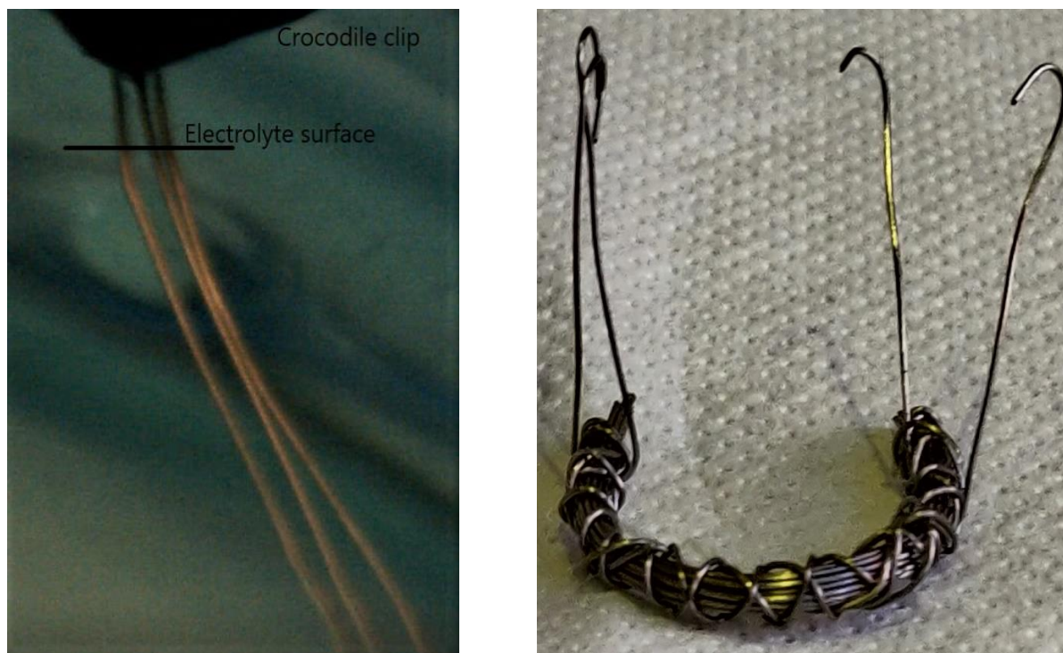
Figure 3-3 Connections for left) three titanium wires; right) titanium wire bundle
