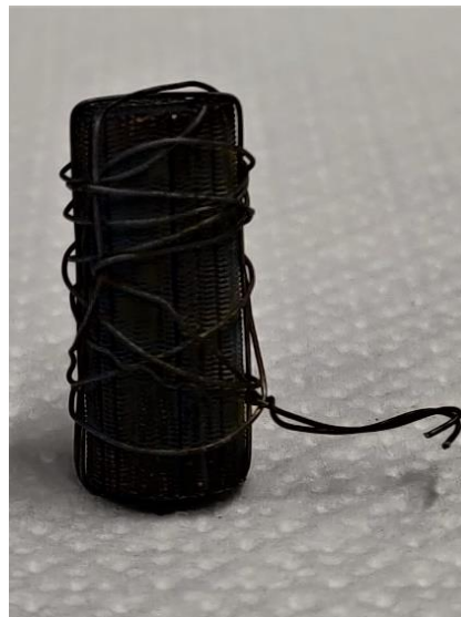
Figure 3-5 Wound 3D printed titanium scaffold sample
