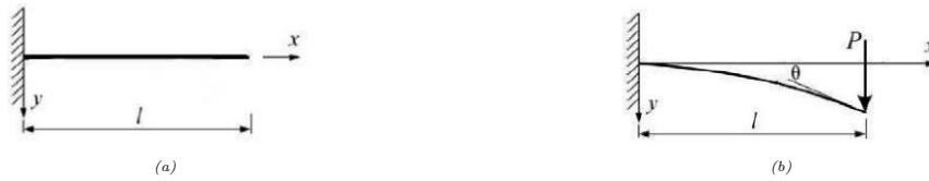
Figure 2.6: (a) Cantilever beam, fixed on one end and free on the other end [7], (b) Cantilever beam subjected by a point load P [7]
