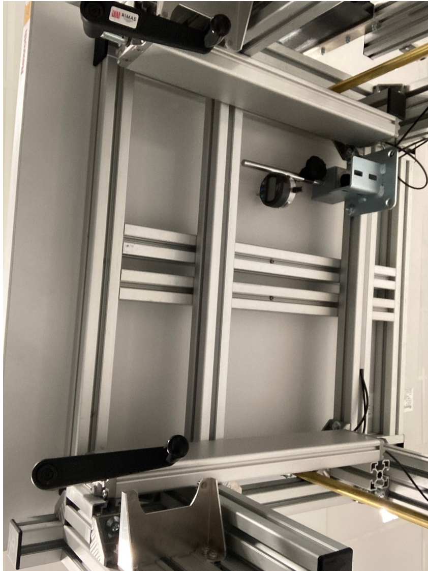
Figure A.12: Placement of the DI underneath the tabletop.
