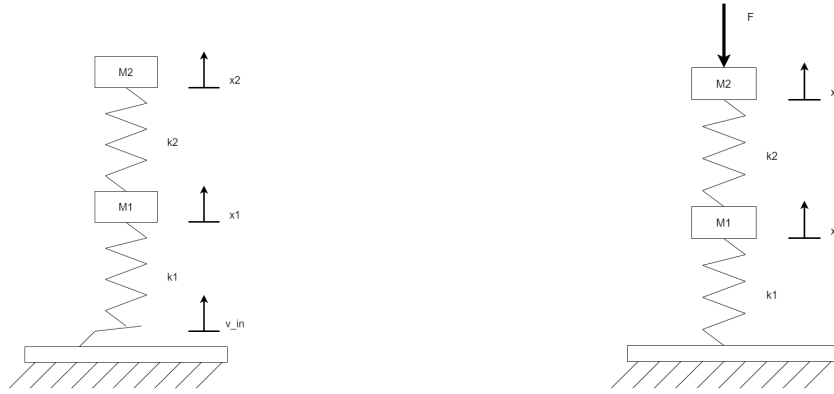
(a) Representation of the lumped mass model with the floor vibration as input. (b) Representation of the lumped mass model with the reaction force as input.
