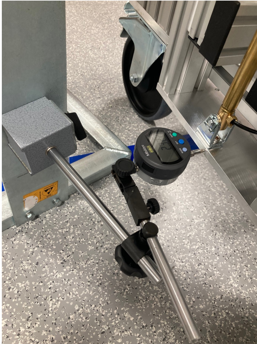
Figure A.8: Placement of the DI for the measurement of the wheel stiffness.
