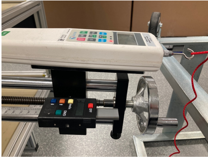
Figure A.9: Spindle used to hold the force gauge and apply tension on the wire
