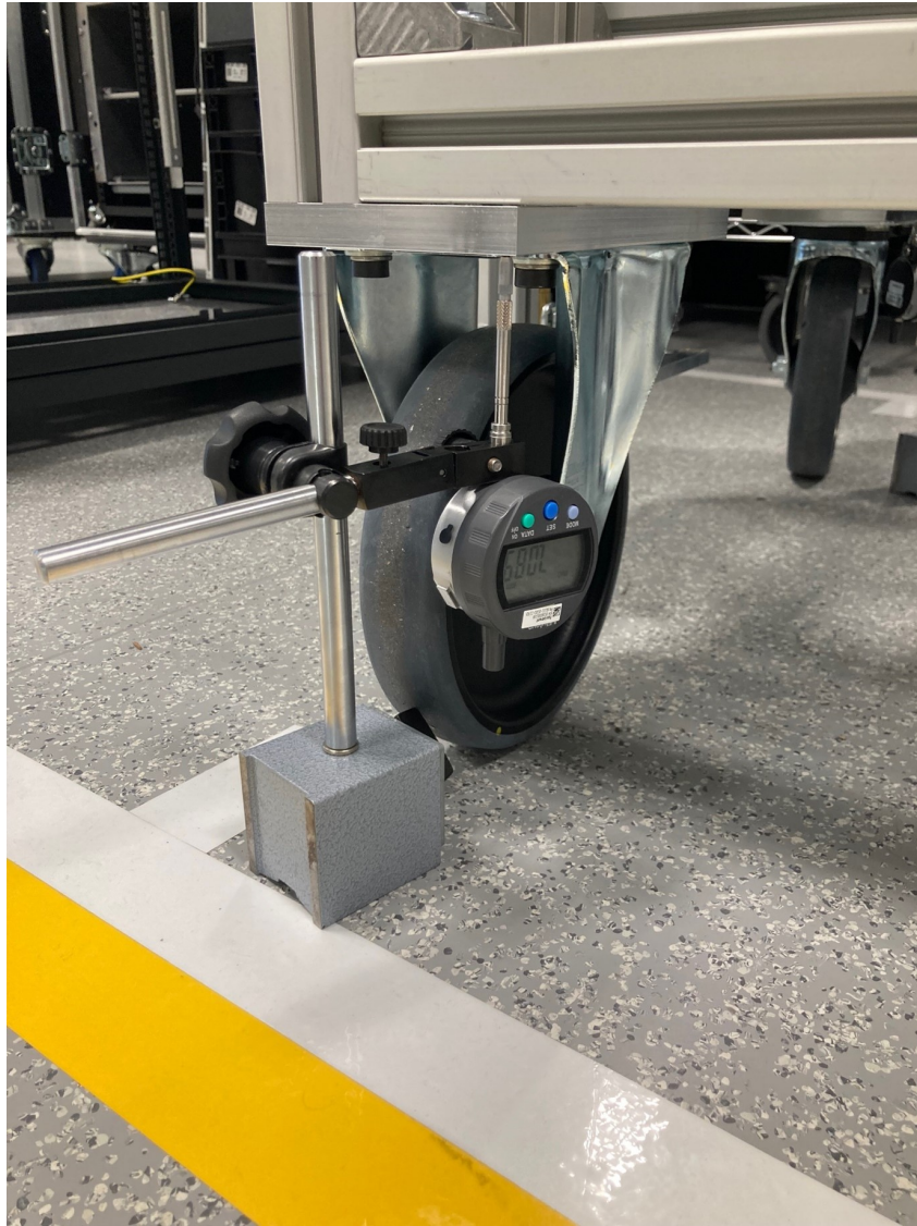
Figure A.14: Placement of the DI at the wheels.
