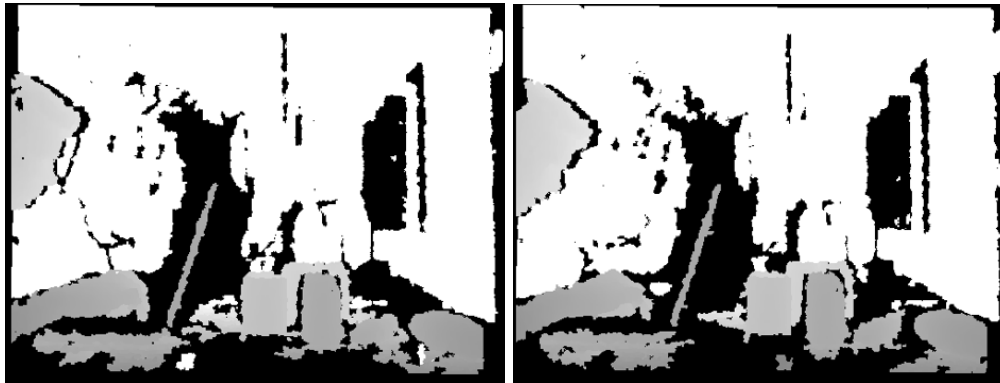
Figure 18: Extracted depth information displayed for 2 images, black refers to unsuccessfully measurements, grey/white sections contain depth information where the intensity is determined by the range
