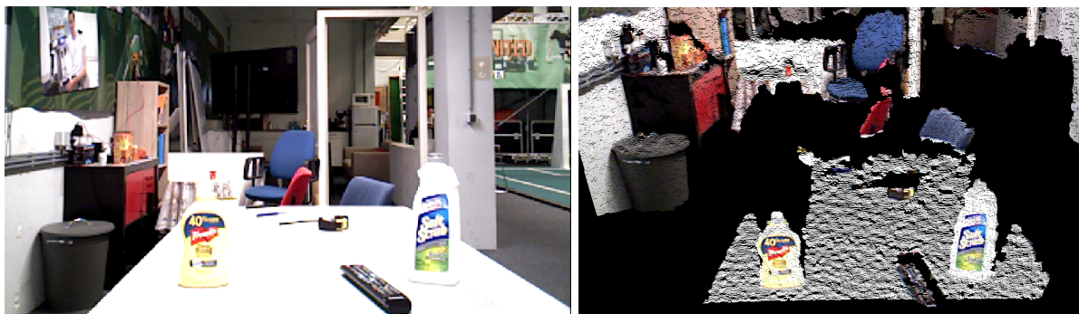
Figure 3: Common RGB image compared to an image including additional depth information, where the black sections in the RGBD image represent space that is not visible from HERO's point of view
