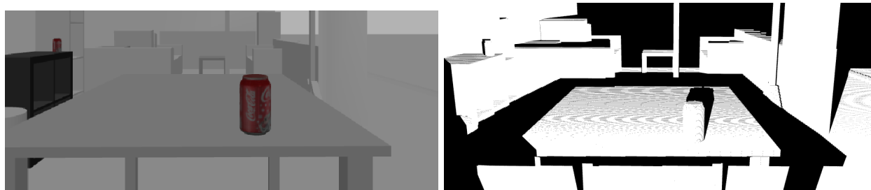
Figure 9: The situation as seen in the RGB image and the depth information that is extracted on the right
