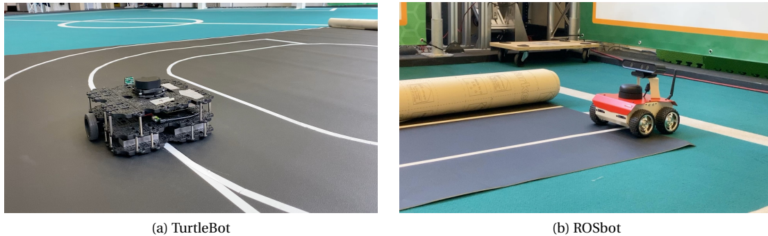
Figure 6.18: Pictures of the line follower on the TurtleBot 3.0 Waffle Pi and the ROSbot 2.0.
