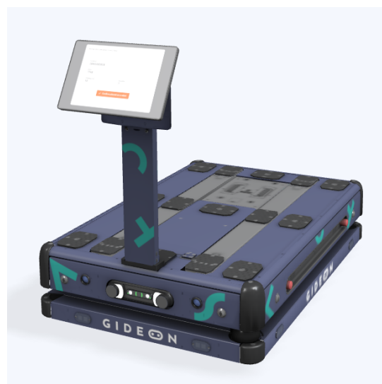
Figure 11. Casey robot developed by Gideon for case picking
