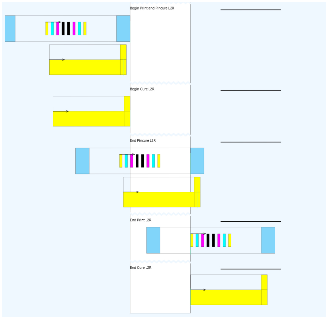
Figure A10: SP DSL model for pin cure motion profile - left-to-right Situations - graphical representation.
