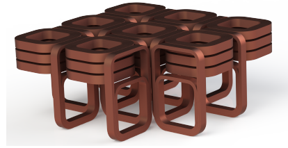
Figure 19: Stacked geometry in combination with convoluted vertically oriented coils.
