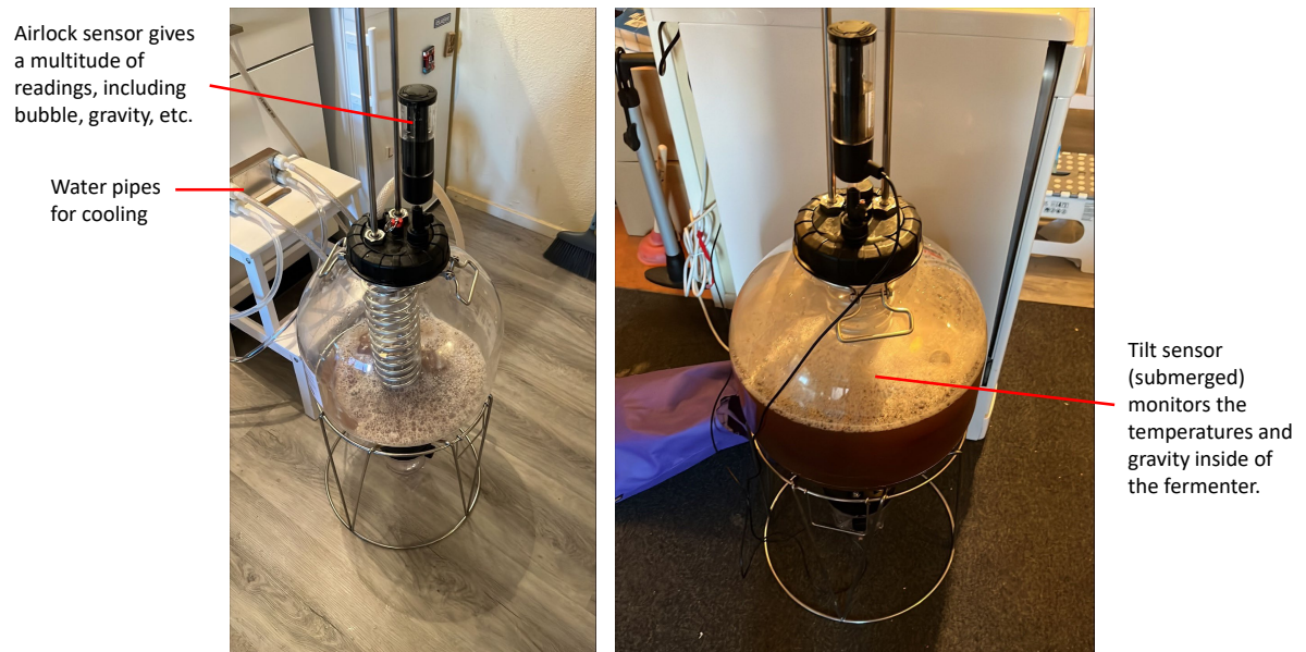
Figure B.1: The fermenter before (left) and after (right) being filled up with wort.
