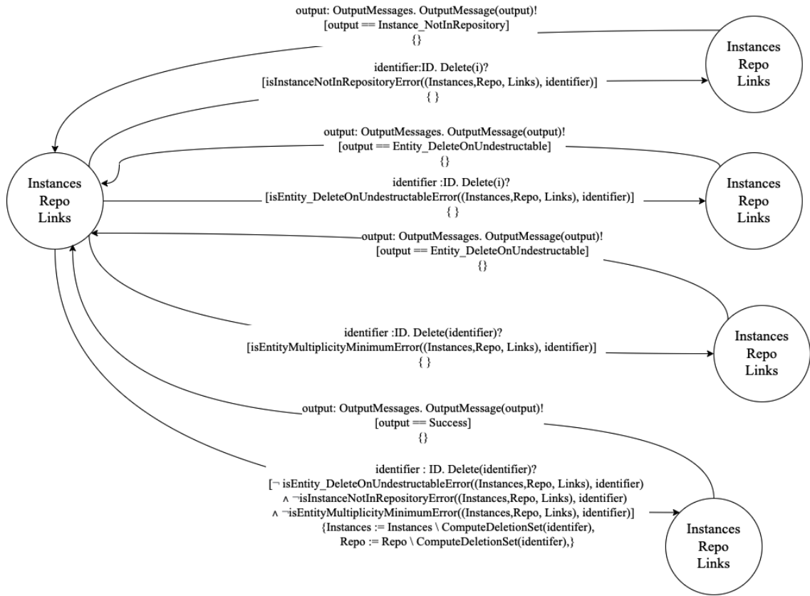
Figure 5.3: Model idea 2 - The dynamic semantics of the delete action of DMDSL represented as STS.
