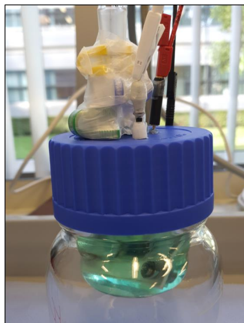
Figure 7 – a) A general schematic of a three electrode cell consisting of a working electrode (red), counter electrode (blue), and a reference electrode (white). b) The enclosed electrochemical cell fabricated by ourselves (setup I). A beaker without a beak was inserted into a flask with cap. The cap was modified to accommodate the three electrodes.
