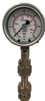
Figure 45: Autoclave with a pressure meter used for measuring the pressures.
