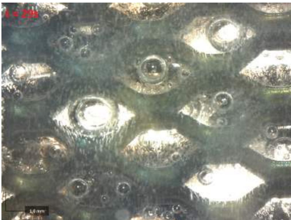
Figure 4.7: Front electrode is cathode and back electrode is anode. The backside of the cathode over time where t = 0s indicates the moment the current is switched on at a current density of 6.7 \text{ mA/cm}^2 . Pictures are taken at 0, 9, 13 and 29 seconds after switching on the current from top to bottom. A bubble size measurement is included at 13 seconds.
