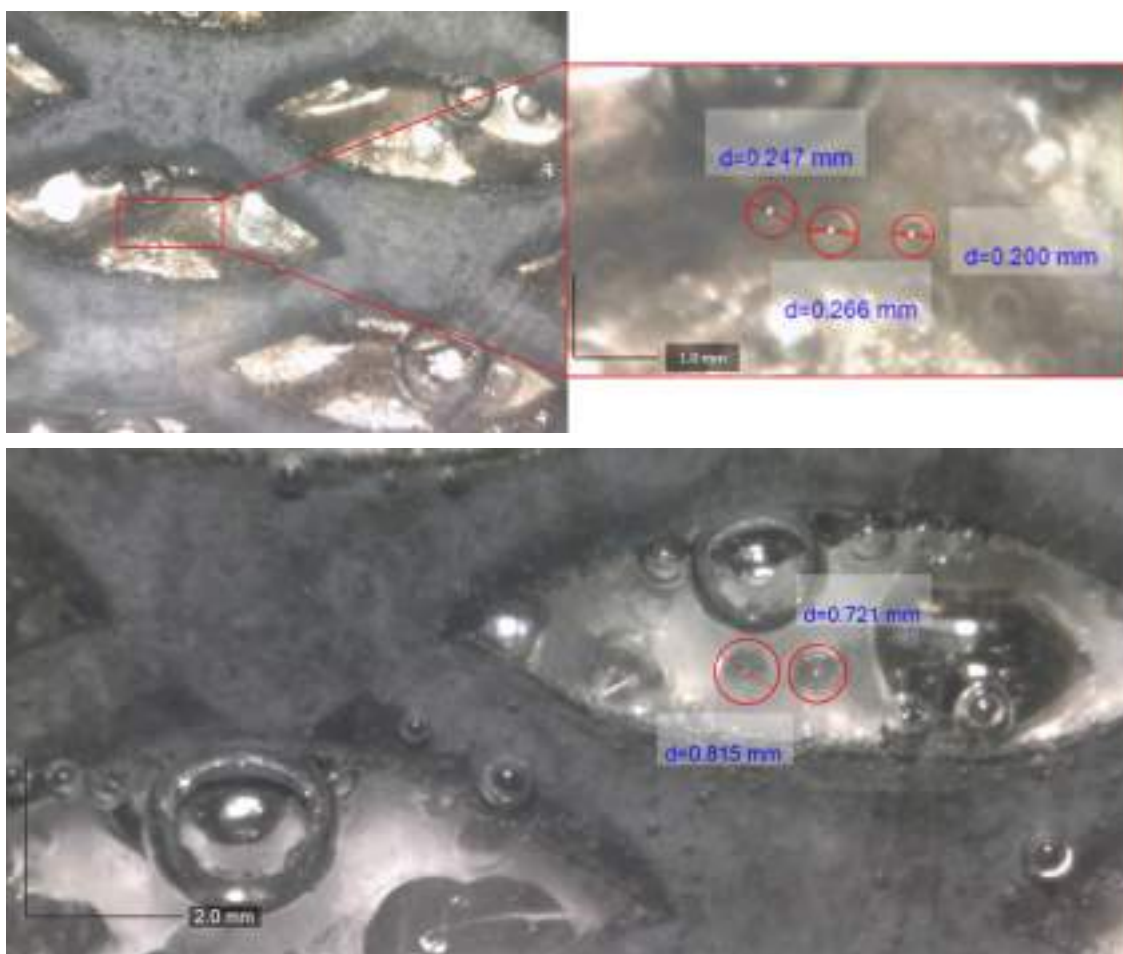
Figure 4.2: Front electrode is anode and back electrode is cathode. Static bubbles reaching a diameter of around 0.2 - 0.3 mm during operation at a current density of 6.7 mA/cm 2 (top) and static bubbles reaching a diameter of around 0.7 - 0.8 mm at a current density of 300 mA/cm 2 (bottom). Both pictures are taken at different positions of the electrode.
