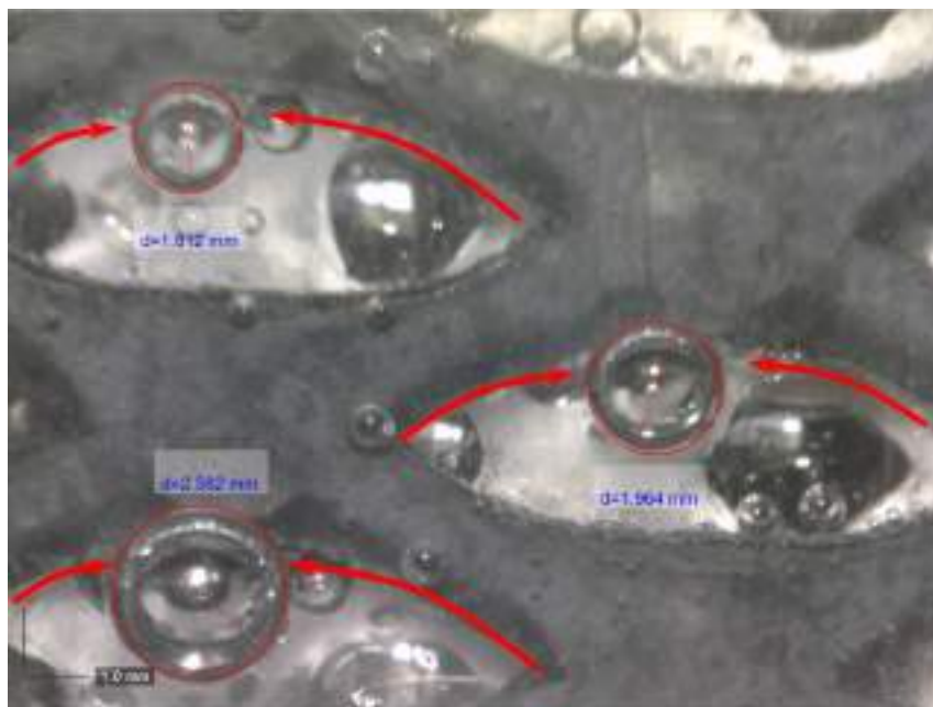
Figure 4.9: Front electrode is anode and back electrode is cathode. The sliding direction of the bubbles is indicated with the arrows and the large bubble formed due to coalescence is indicated with the ring around it.
