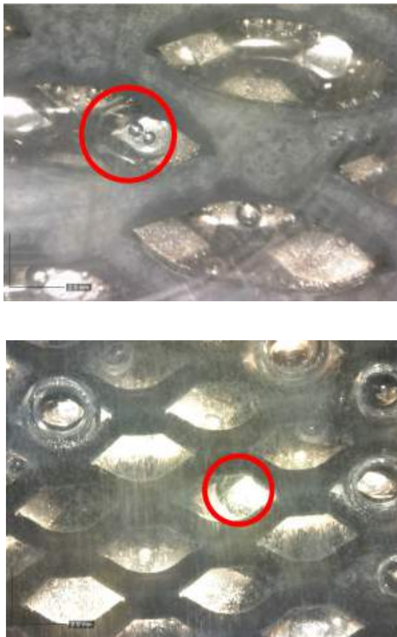
Figure 4.5: Gas pocket left behind by large bubble after detachment seen from anode (top) and seen from cathode (bottom)
