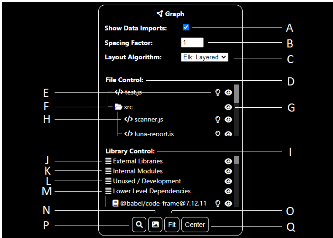
Figure 3.10: Graph menu in LUNA's generated report. Menu elements: A) Toggle visibility of all the JSON data files that are imported; B) Change the distance between nodes via this spacing factor; C) Change the positions of the nodes in the graph dictated by the selected layout algorithm; D) The section to control all the file nodes that exist in the graph; E) Toggle highlighting of a node in the graph; F) A folder that is collapsible (via double click) in the file control section; G) Toggle visibility of a node in the graph; H) A file in the file control section; I) The section to control all the library and dependency nodes that exist in the graph; J) External libraries group; K) Internal libraries group; L) Development libraries group; M) Dependency graph group; N) Take a screenshot of the graph that is in the viewport and save it to disk as 'luna.png'; O) Fit the whole graph into the viewport; P) Search for a node in the graph by label (case-insensitive); Q) Reset the position of the viewport to the center.
