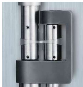
Figure 26: Example of uniaxial extensional measurement rheology tool for a rotational rheometer.
