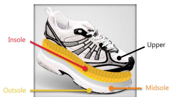
Figure 1: Different components of the soling in athletic footwear.
