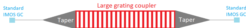
Figure 2.7: Schematic illustration of the large grating coupler structures on the TU/e test PIC. It consists of two standard IMOS grating couplers at the input and output (blue), which are connected to waveguides (light grey). The guided mode is expanded into the large grating coupler (red) through a taper (dark grey).
