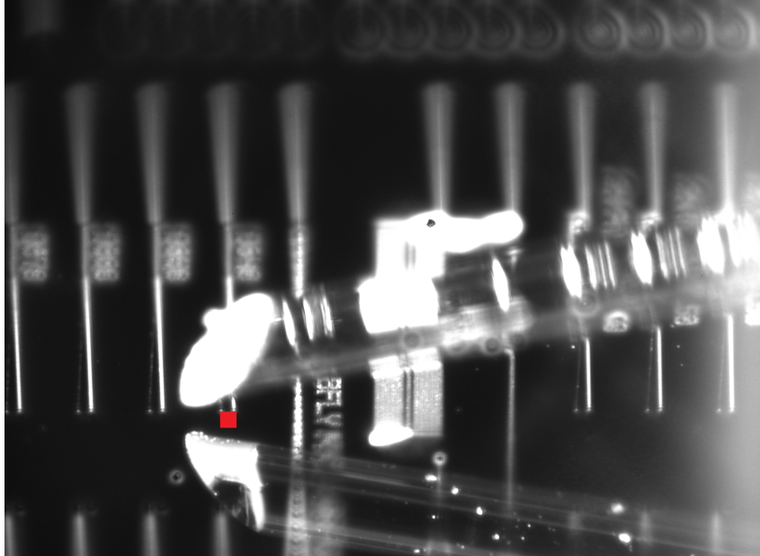
Figure 5.4: An image, captured by the visible light camera system, of the optical fiber in the aligned position. The fiber (top) is brought close to its reflection (bottom), above the standard IMOS grating coupler (red square).
