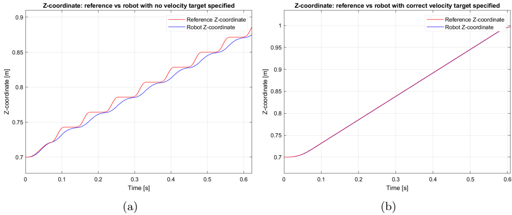
Figure 4.8: (a): Generated reference signal with zero velocity at each waypoint. (b): Generated reference signal with correct velocity at each waypoint.
