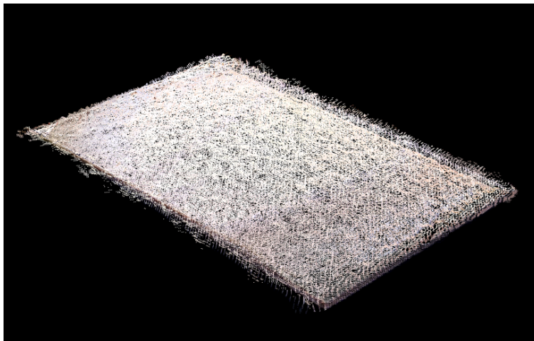
Figure 6: The result of applying iterative closest point, note that the edges are slightly more defined than in Figure 4
