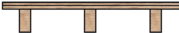
Figure 17a: Cross-section of the ground floor for the uninsulated floor and the variants with insulation on the bottom of the crawl space
