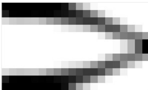
Figure F.9: Optimized topology of cantilever beam problem at iteration 21
