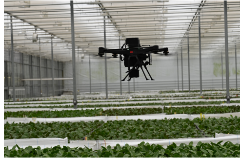
Figure 1: An autonomous quadrotor inside a greenhouse used to monitor plant health and growth.
