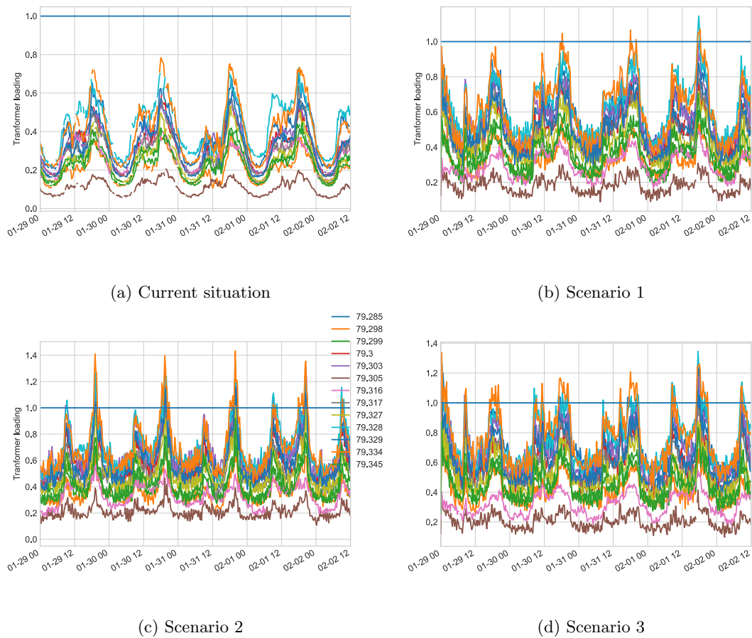
Figure B.1: Power loading of all transformers with heat pumps but no Electric Vehicle. The simulation was done for the entire month of January and February. A snapshot of 29th of January to 2nd of February 12:00 is shown because this was a fairly congested period when the simulation was executed.
