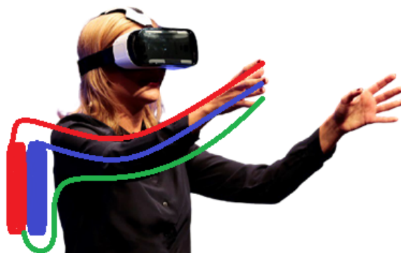
Figure 2.3: user sketched with liquid setup, (red) hot fluid feed line, (blue) cold feed line, (green) return line
