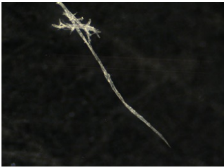
Figure 2-3: Single paper fiber before wetting.
