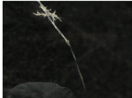
Figure 2-4: Single paper fiber 10 minutes after wetting.
