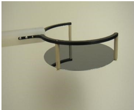
Figure A.6: An example of a gravity/friction force based handler for thin wafer handling
