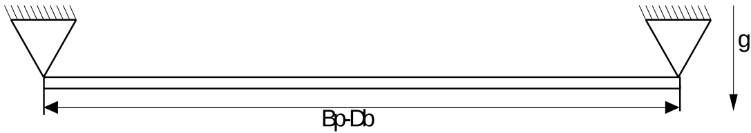
Figure 3.6: A schematic of a wafer section, simply supported on both ends
