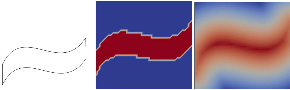
Figure 3.8: Original geometry (left), the sign function (middle) and the signed distance function (right) as levelset functions
