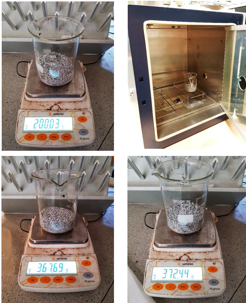
Figure 4.12: [Top Left] 200 g sample after taring the weight of the beaker [Top Right] The sample is placed in the convection heater for 24 h at 100 °C [Bottom Left] The weight of the dehydrated sample + beaker (173 g) is 367 g [Bottom Right] After 24 h, the weight of sample + beaker (173 g) is 372 g. This shows that during overnight cooling, the sample absorbed 5 g of H 2 O.
