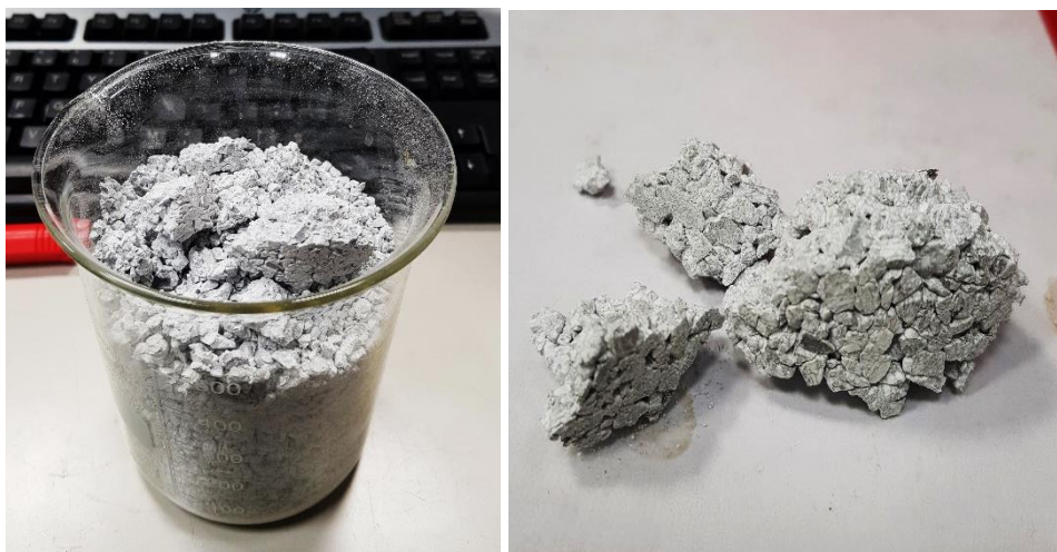
Figure 4.25: Agglomeration of the K_2CO_3 composite at the end of an experimental phase
