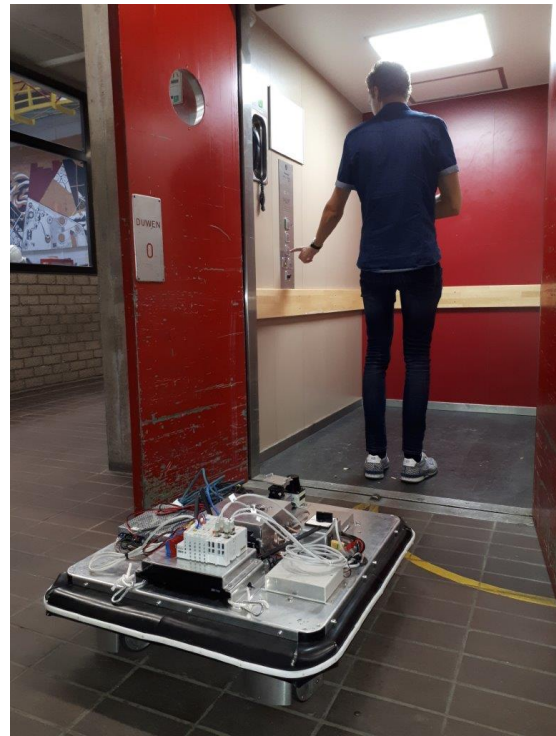
Figure 2: The ropod platform wants to enter the elevator. With the laser, the ropod measures that it will not fit and therefore the ropod will not attempt to enter it. In reality the robot can “squeeze” itself in the elevator and the person will step aside.
