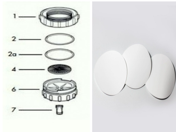
Figure 5.4: Filter holder parts (left) and PVDF membrane disc(right)
