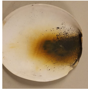
Figure 5.5: Particles collected over the edge of the membrane filter
