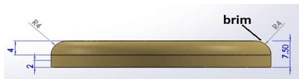
Figure 3.1: Lower electrode new design (sizes are in mm)
