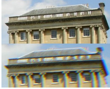
Figure 2.13: An illustration of the two chromatic aberrations from [22].
