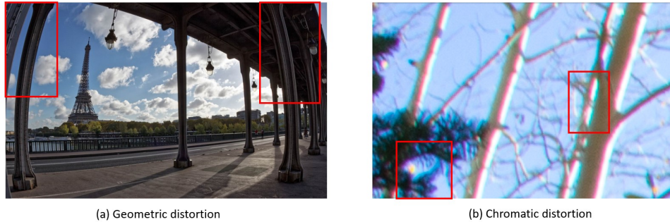
Figure 1.1: Representative aberrations exist in photographs. (a) Geometrical aberration [4]. (b) Chromatic aberration [5].
