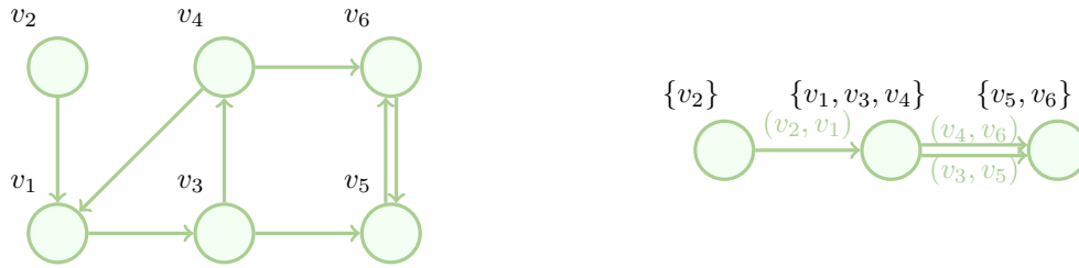
Figure 6.2: The graph on the right shows visualisation of the effect of the function condense(G) , on the graph on the left
