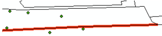
Figure 1.2: An example trajectory influenced by multipath errors. The trajectory consists of 6 green dots and the road segment marked in red is where the sensor actually passed.
