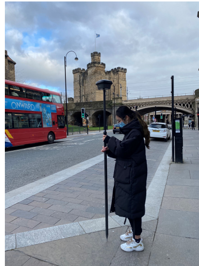
(b) Use Leica GS18 T to collect position data.
