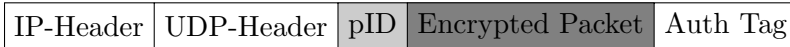
Figure 4.1: Structure of a PQConnect packet with the tunnelID , Epoch No., and Packet No. replaced by the secure pID header: Light gray areas are authenticated but not encrypted. Dark gray is authenticated and encrypted
