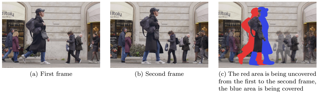
Figure 5.2: Frames from a video showcasing occlusion.
