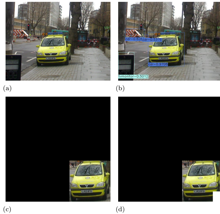
Figure 4.2: Example of a car that has been cut out according to its bounding box and pasted in the bottom right corner of a black background, both without and with backdoor pattern
