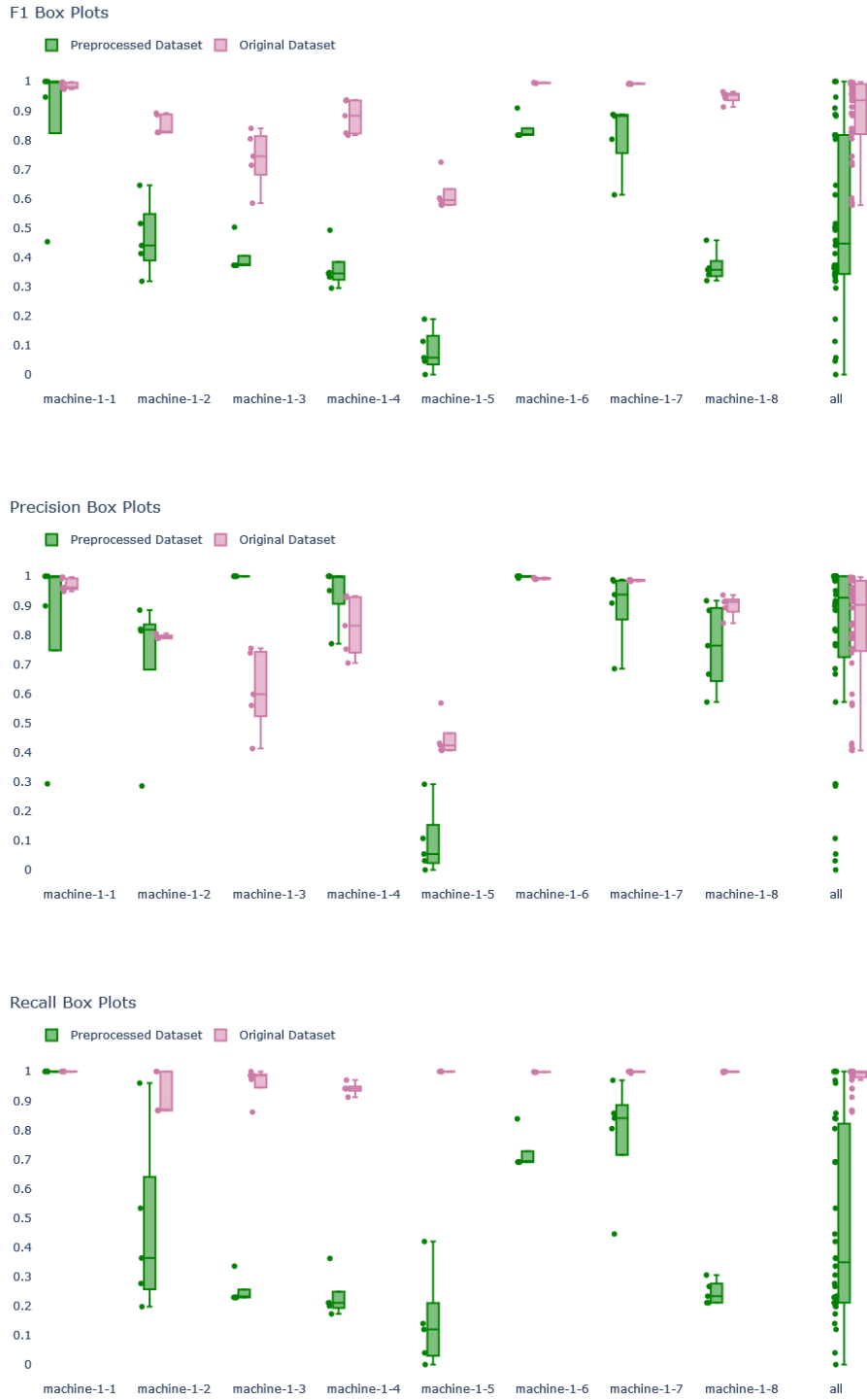
Figure 22: Anomaly detection performance: precision, recall, F1 box plots for 8 machines' preprocessed (green) and original (pink) datasets, each with 5 runs.
