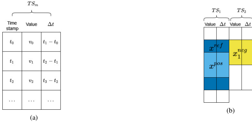
Figure 5: (a) An example of obtaining \Delta t column from the timestamp column for a sensor m . When encoding the data, only value columns and \Delta t columns are used. Timestamp columns are discarded. (b) Time-based sampling with \Delta t .
