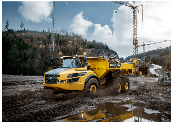
Figure 2.3.1: Articulated Hauler - A40G Series (Image retrieved from [51])
