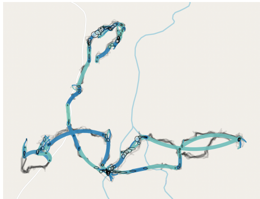
(c) The same segmentation as in (a) now with arcs and with location model ellipses drawn transparently. The ellipses are drawn based on the parameters used in the location models, \sigma_x, \sigma_y .
