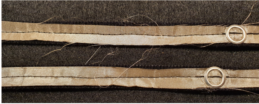
Figure 5.2: A photograph showing the torn threads of the conductive fabric
