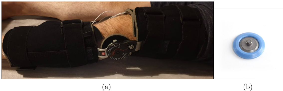
Figure 3.9: (a) Full leg brace used in combination with the dry Non-gelled Ag/AgCl electrodes to ensure better contact with the skin. (b) A photograph of the used dry electrodes.
