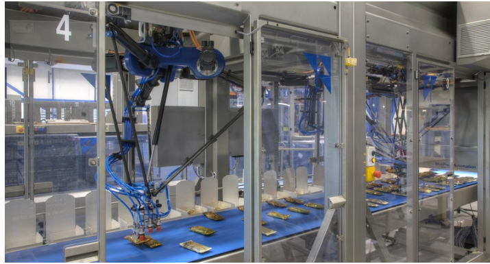
Figure 1.1: Double Spider DPR01 setup, BPA
