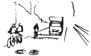
Image 6: In shared streets, cars have to adapt to the speed of slower traffic. The design of the street can slow down fast bicycles as well.
