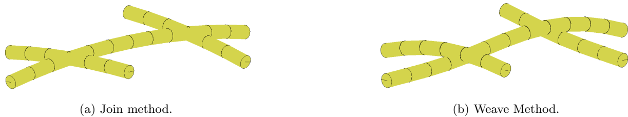
Figure 1.2: A close up of two cross-over points in a beam element model using the join method (a) and the weave method (b).
