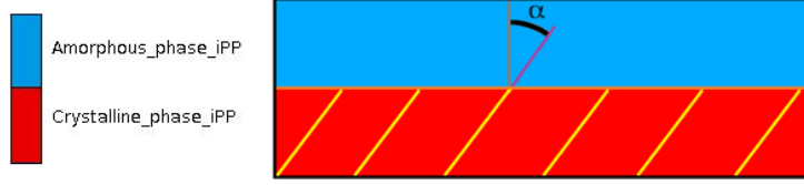
Figure 2.6: Schematic representation of the chain tilt angle in a 2D example. With amorphous material in blue, crystalline material in red, chain direction in yellow, the normal to the fold plane in grey, the fold plane in orange and alpha being the chain tilt angle.
