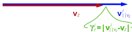
Figure 2.13: Visualisation of a measured velocity vector v_z , a particle's velocity vector v_{||v_z}^i and the measurement residual, \gamma_r^i between them. These are used to calculate w_v^i according to [21].
