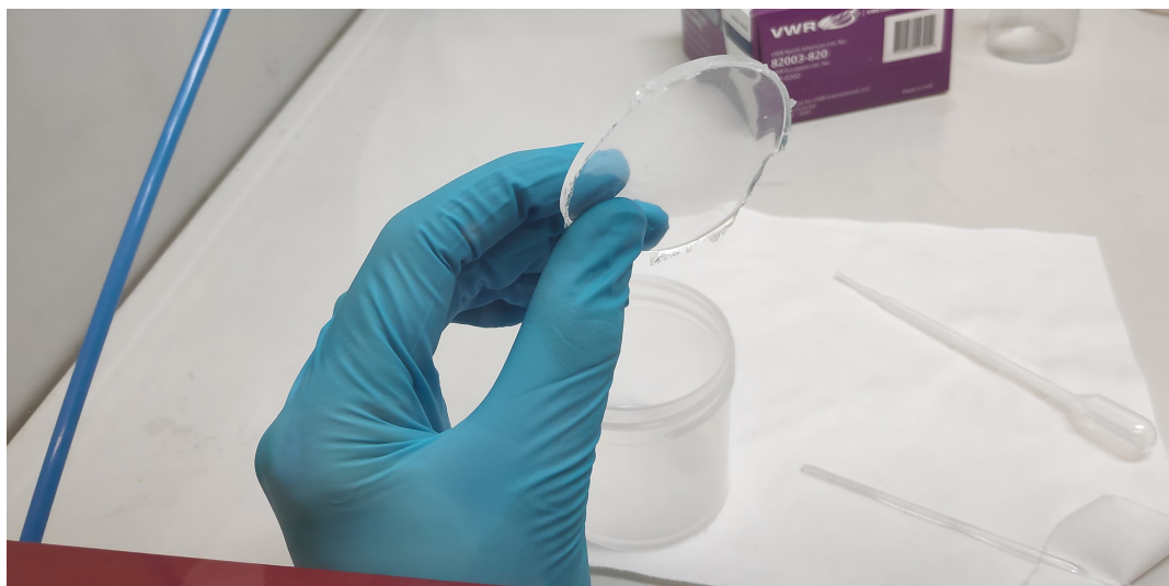
FIGURE 3.5: A fully cured layer of PDMS. It is transparent and by the refraction of my finger, the refractive index n = 1.4 becomes apparent.
