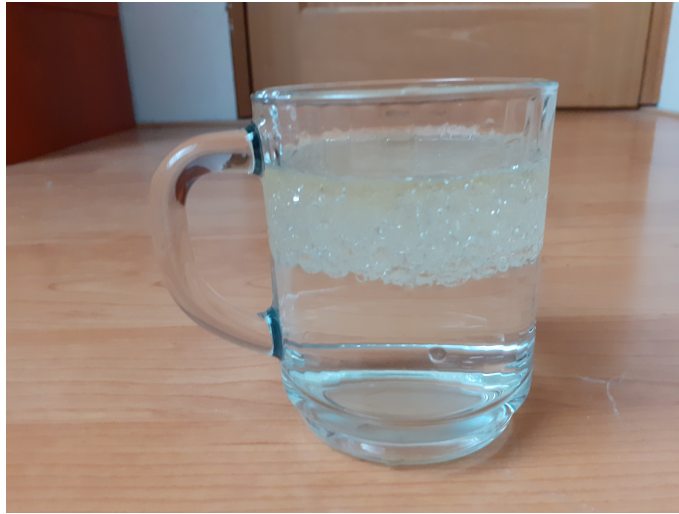
Figure 2.2: Example of an oil-in-water emulsion after stirring with a tablespoon. The droplets can be seen to be nearly spherical and do not immediately coalesce despite nearly touching one another due to the inertia still present in the system at the time this picture was taken.
